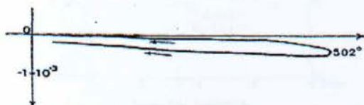
FIG. 46.—Duralumin compared with pure Aluminium, using Dilatometer.
