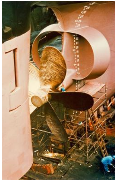
Figure 5.18 Typical wake equalising duct
