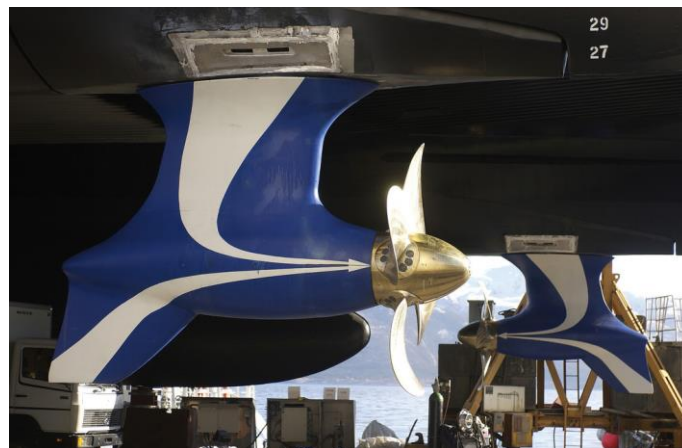
Figure 5.26 Azipull Pulling thruster
