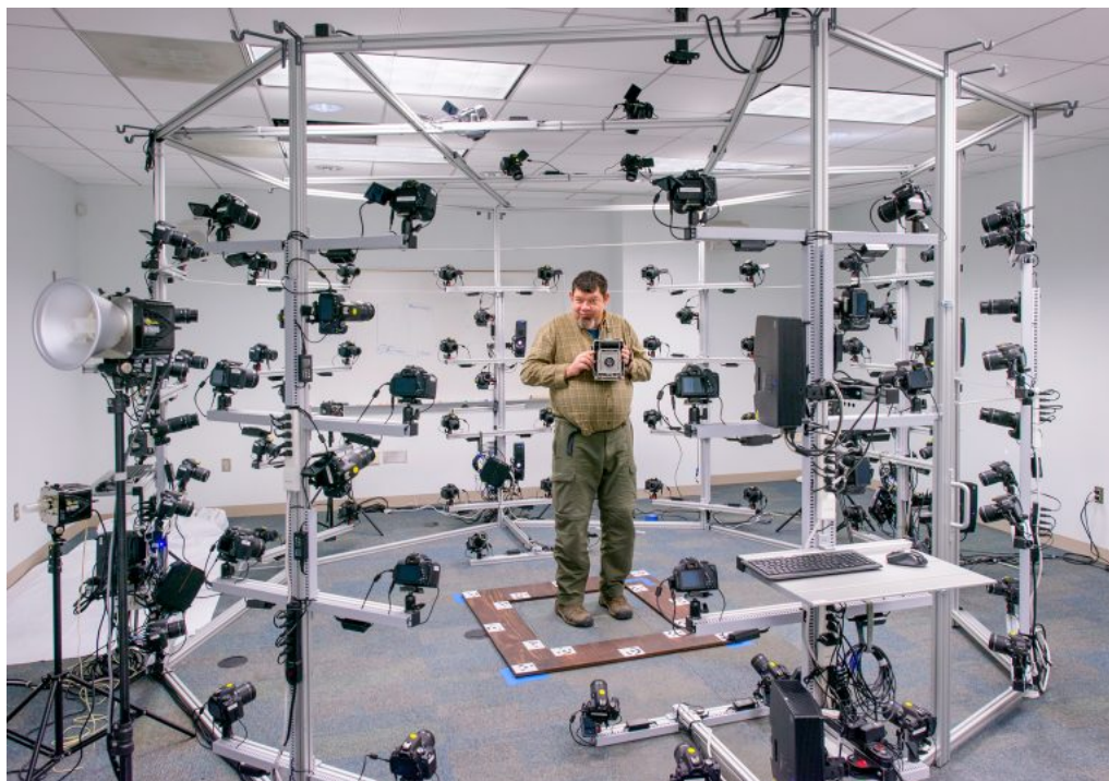
Σχήμα 2.18: Chris Perego along with his antique camera, is being 3D scanned in the newly installed 90 digital camera rig. Imaging Research Center UMBC.
