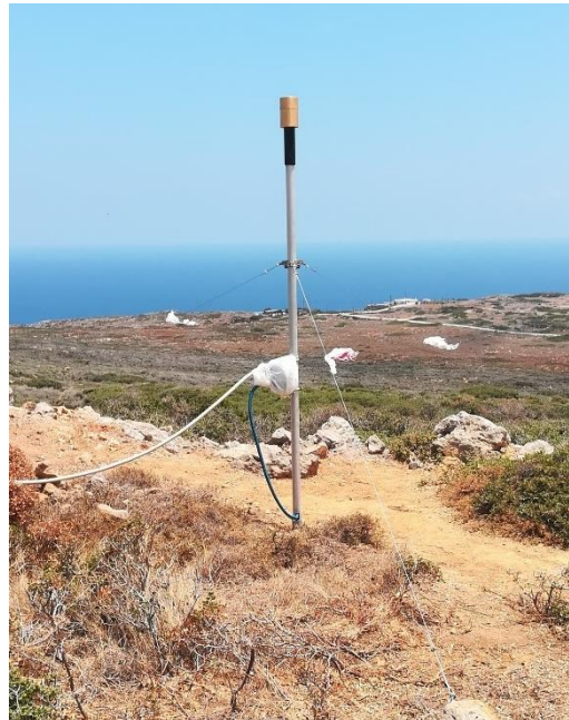
Figure 23: Photo of the Electric Field Mill at the Antikythera Observatory. The instrument has been since moved to another part of the island.
