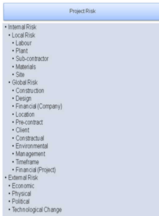
Figure 2: Hierarchical Risk Breakdown Structure (J. H. M. Tah & V. Carr, 2000)
